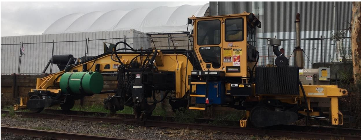
Figure 3 (Tripp Machine) – Nordco Tripp machine (16.4 tonne)
