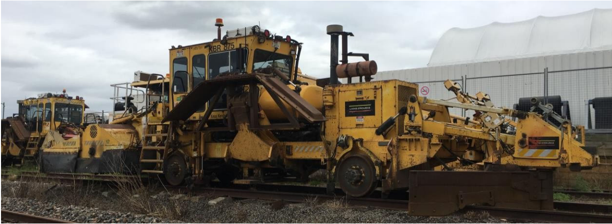
Figure 1 Track Machine - Kershaw KBR 875 Ballast Regulator (18.5 tonne) / Kershaw KBR 925 Ballast Regulator (20.5 tonne) / Tripp Machine (16.4 tonne)
