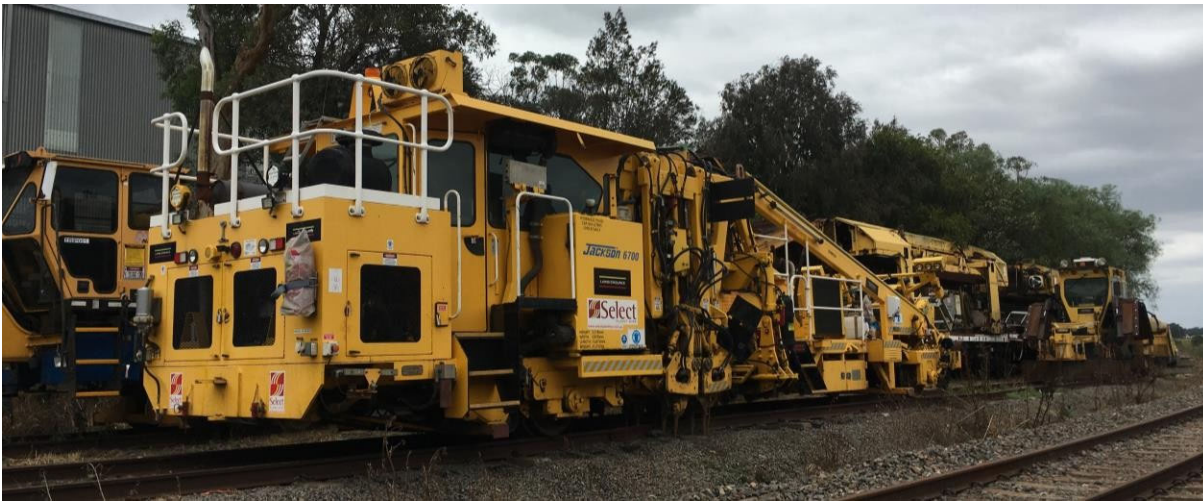
Figure 2 (Tamper) – Jackson 6700 Tamper (32.5 tonne) / Jackson 6700S HTT (32.5 tonne) Tamper
