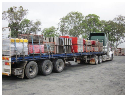
IMAGE 4 - Good practice – can be removed by Forklift or Crane with suitable platform provided by the Project / Workplace
