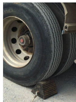
IMAGE 5 - Wheel chock in place
