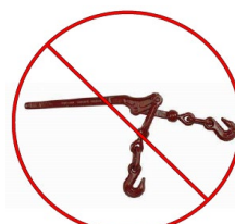
IMAGE 8 - Spring load chain binders are not to be used
