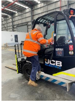
Photo 1 - Climbing into forklift maintaining three points of contact.
