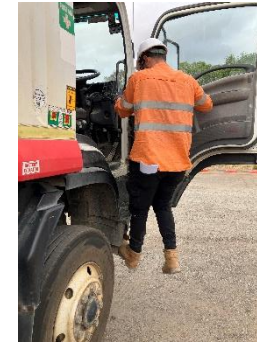
Photo 2 - Climbing into the truck maintaining three points of contact.
