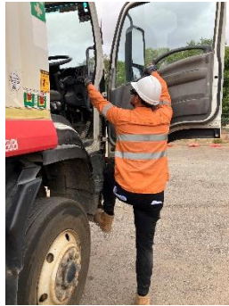
Photo 1 - Climbing into the truck maintaining three points of contact.
