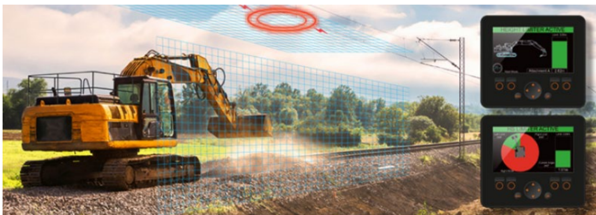
Excavator with Height and Slew Restrictors
