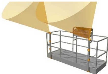
Example - Proximity Systems - Secondary Guarding System
