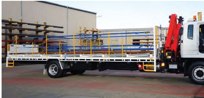
Example of a good webbing type edge protection system
